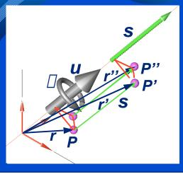
■ The sequence is shown by the fact that [R] operates on the displaced **r** after it has had **s** added to it
