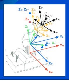
For instance, we probably want to be able to describe where objects are in terms of a convenient world coordinate system fixed in the robot's base.
