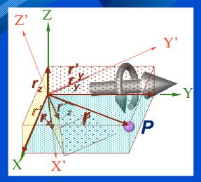
■ We wish to determine a coordinate transformation matrix [T] that will leave the point P in its original position but rotate the coordinate system.
