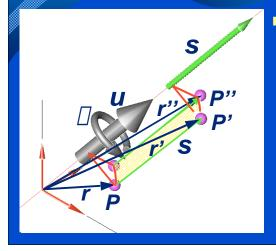
Notice we end up in the same place since we have done something akin to forming a parallelogram on the surface of a cylinder
