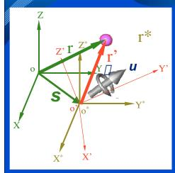
■ We want to find the components of **r'** in the translated and rotated coordinate system, knowing the original **r**
