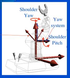
Then the shoulder pitch angle is all we need to know in order to figure out where the shoulder is with respect to the blue system.
