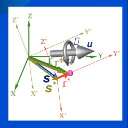
A typical point P is defined in the current coordinate system x' y' z' by position vector r'.
