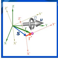
■ Given the point P in the original system located by **r** we want to find the components of **r**'
