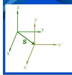
■ After translation by vector **s** we are brought to the coordinate system x\* y\* z\* as shown:
