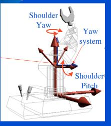
The blue system's position relative to the world system is completely specified by the shoulder yaw angle variable and the offset along the z axis which is a constant.
