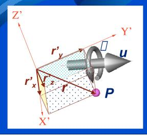
■ In the new coordinate system, it has the components  $r'_x$ ,  $r'_y$ , and  $r'_z$ .
