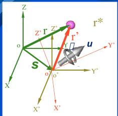
Step 2: Rotate x\* y\* z\* by [T] matrix:
