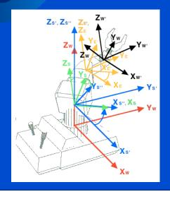
As you go across a joint, an easily written 4X4 transformation matrix (which is a function of the joint variable) can bring us from the coordinate system on one side of the joint to the one on the other side.
